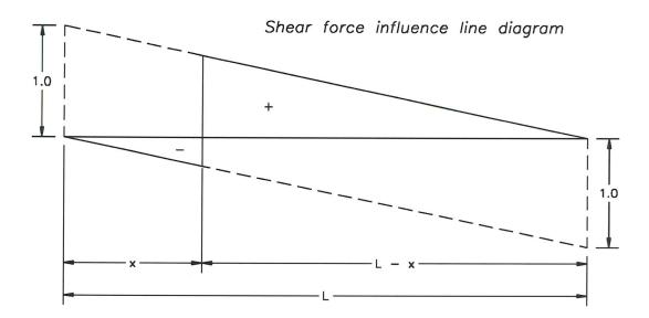
The shear forces at any point x from one end are represented by the areas of the positive and negative triangles in the diagram above and are tabulated below.
