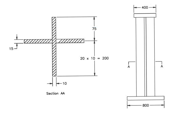
The width of the stiffeners, chosen to come within the width of the top flange will be taken as 150 mm.
