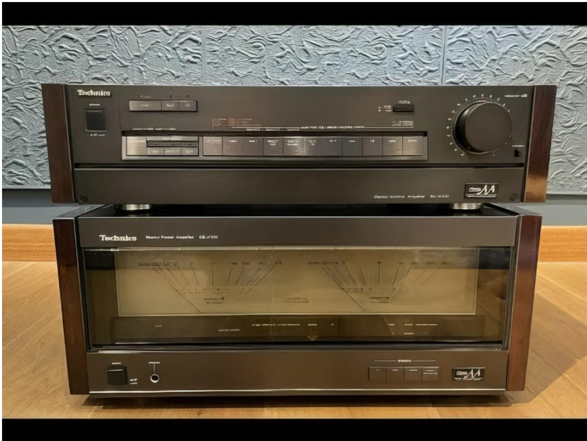
During the late 80s, this was Technics stunning flagship pre-power amp combo. The SEA-100 power with the SUA-200 pre.
