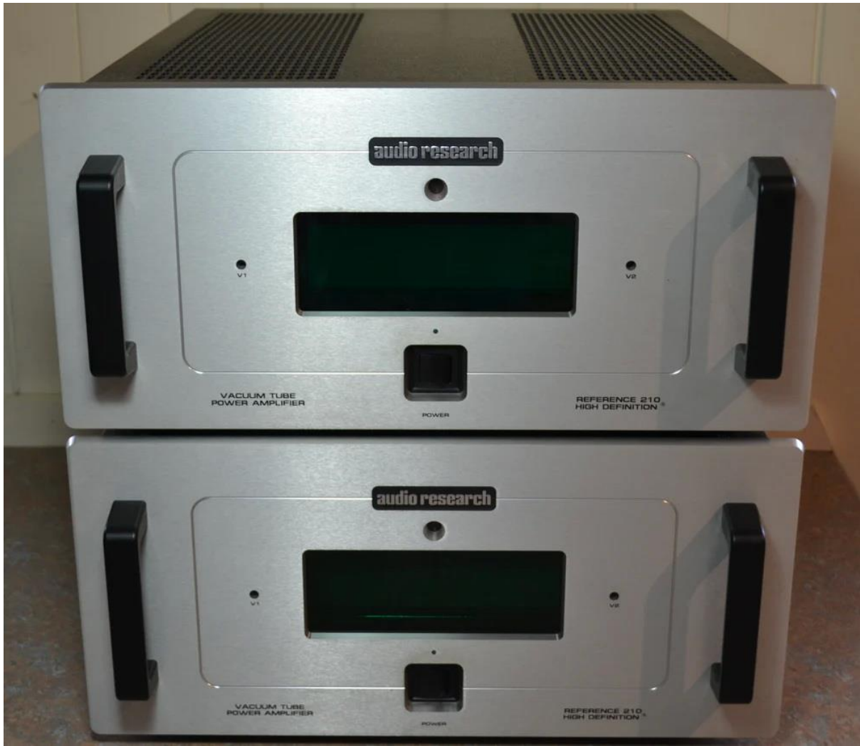
Audio Research valve-driven monoblock power amplifiers
